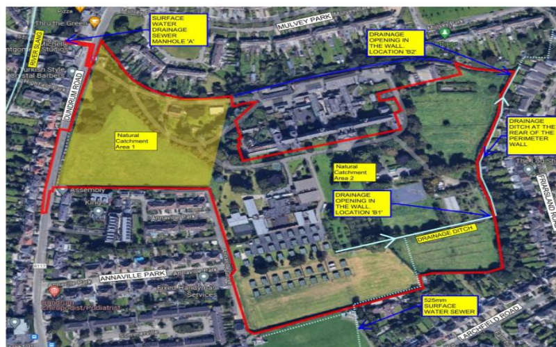
Fig 3.1. Aerial View of the Approximate Natural Catchment Areas and surface water drainage outfalls on the Existing Site. Catchment 1 shaded yellow. Catchment 2 is in the unshaded area.
